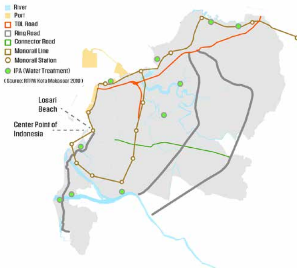
Figure 16. The City of Makassar has a number of infrastructure development projects planned as part of their vision including: a ring road, expansion of the port facilities, a new monorail system, water treatment plants and new developments along the coast. As the city grows such new infrastructure becomes necessary, but new developments can also affect human vulnerability to climate change for example by displacing fishing communities and altering some of the local economies upon which they rely for their livelihoods.
